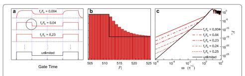
**Figure 9 Bandlimited filters.** Effect of bandwidth limits on Walsh filters. (**a**) Bandlimited reconstructions of WAMF $_{0.3}^{(1)}$  modulation envelope as a function of first-order Butterworth filter parameter  $f_c/f_s$ . (**b**) *Red*: Closeup of circled region in (a); *Black* ideal square profile. (**c**) Filter-transfer functions for profiles in (a).
