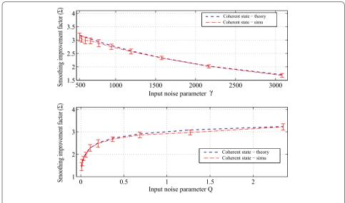
Figure 6 Smoothing improvement factor  $(\Sigma)$  for a coherent state for varying input forcing function  $(S_f(\omega))$  parameters Q and  $\gamma$ .
