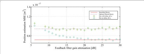
Figure 9 Mean square position error for both experiment and simulator as a function of feedback gain.
