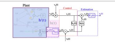
Figure 3 The block diagram with additional gain block used for the derivation to recast the smoother as a position estimator. Here the transfer function h(t) is modified to h'(t) that assumes position,  $x_e(t)$  (units of metres), rather than voltage,  $v_e(t)$ , as an input. As such the smoothed output,  $x_s(t)$ , is similarly a position estimate.
