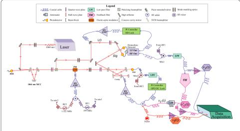
**Figure 7** The full experimental setup for the coherent state cavity mirror position estimation. Note mode cleaning cavity (MCC) locking circuitry is omitted.
