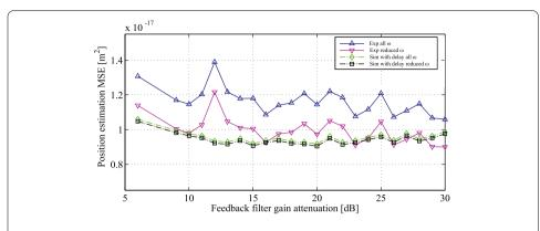
Figure 8 The actual MSEs (blue triangles and green diamonds) and the frequency truncated MSEs (pink inverted triangles and black squares) in position for both experiment and simulator as a function of feedback gain.
