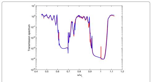
Figure 8 Transmission spectrum the quantum metamaterial in the absorption regime (in blue) and in the emission regime (in red). The peak corresponds to the transition of the quantum dots.
