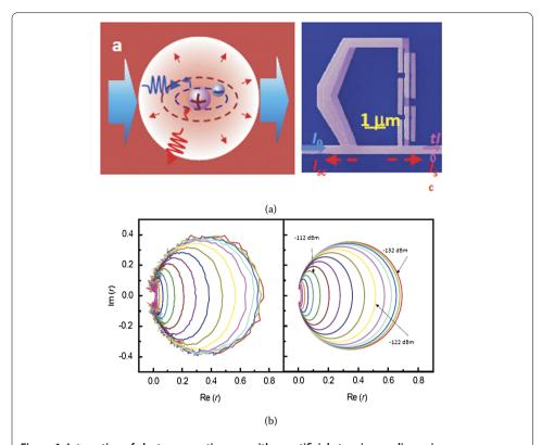
**Figure 1 Interaction of electromagnetic wave with an artificial atom in one dimension.**(a) A 'proto-metamaterial': a single artificial atom (flux qubit) in a transmission line. (b) Reflection coefficient of a microwave signal in the line measured (left) and calculated (right) for the structure of (a). After Ref. [34].
