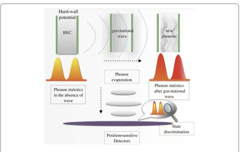
Figure 1 Sketch of the setup: A BEC in a box-like potential that acts as a cavity for the phononic excitations. Two phononic modes m and n are initially prepared in a thermal two-mode squeezed state represented by the initial covariance matrix  $\sigma_0$ . A gravitational wave of amplitude  $\epsilon$  transforms the state producing excitations. The new state  $\sigma_\epsilon$  depends on  $\epsilon$ . Measurements on the modes can be used to estimate the amplitude of the spacetime distortion.
