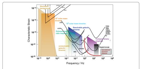
Figure 4 Scaling of the strain sensitivity of our system (solid red line) as a function of frequency in comparison with other gravitational wave detectors (solid black lines).
