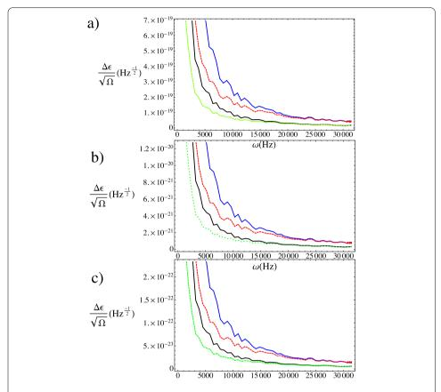
Figure 3 Optimal bound for the strain sensitivity as provided by the QFI vs frequency for t=10, n=1, m=2, T=0 (blue, solid), T=150 nK (red, dashed), m=6, T=0 (black, solid), T=150 nK (green, dotted) and (a) r=5, (b) r=7, (c) r=9.
