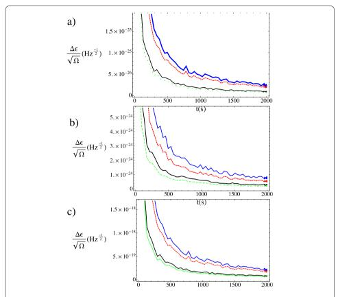
Figure 2 Time evolution of the optimal bound for the strain sensitivity as provided by the QFI for n=1, m=2, T=0 (blue, solid), T=150 nK (red, dashed), m=6, T=0 (black, solid), T=150 nK (green, dotted) and (a) r=10,  $\omega_1=5\cdot 10^3$  Hz, (b) r=10,  $\omega_1=5\cdot 10^2$  Hz, (c) r=2,  $\omega_1=5\cdot 10^3$  Hz.
