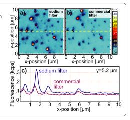
The line cuts in Figure 3(c) illustrate the background level. The image background acquired with atomic filtering is higher by a factor of 7-8 based on a laser-power of 1  $\mu W$  into the microscope. This is fully consistent with the measurements of the optical density: The commercial filter shows an optical density of about seven, whereas the atomic vapor cell was determined to show six orders of magnitude optical suppression.
