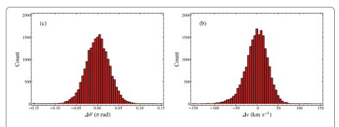
**Figure 8** Matched-filter technique parameter estimation. Histograms of the difference in extracted and injected event parameters from parameter estimation routine. *Left*: Incident direction angle  $\theta$ , resolution of  $\pm 0.05\pi$  radians. *Right*: Event velocity v,  $1\sigma$  resolution of  $\pm 27$  km s<sup>-1</sup>
