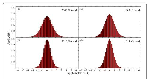
**Figure 2** Signal-free template-specific signal-to-noise ratio distributions. Histograms of template-specific SNR calculations ( $\rho_i$ ) on signal-free simulated data for various clock networks. The network composition for indicated years is given in Table 1. Standard deviations for template-specific SNR values are: 1.15 (2000), 1.03 (2005), 0.86 (2010), and 0.81 (2015)
