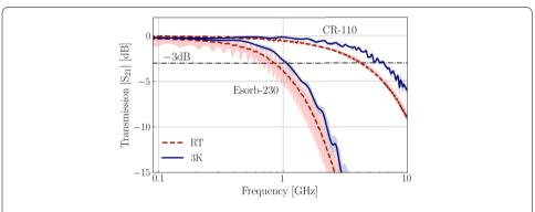
**Figure 4** Low frequency behaviour of filters. –3 dB cut-off frequencies are distinct for both materials and increase when filters are cooled down to 3K
