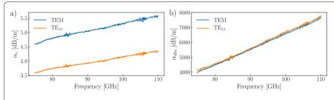
**Figure 12** Attenuation constants of the filter for TEM and TE<sub>11</sub> modes due to (**a**) conductor losses and (**b**) dielectric and magnetic losses in the Esorb-230 material
