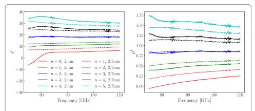
**Figure 11** Real parts of relative dielectric permittivity  $\epsilon'$  and magnetic permeability  $\mu'$  of the Esorb-230 material in the frequency range from 75 to 110 GHz determined by the NRW method. Data for two waveguide section thicknesses d=2.0 mm and d=2.7 mm and different solution branches are shown
