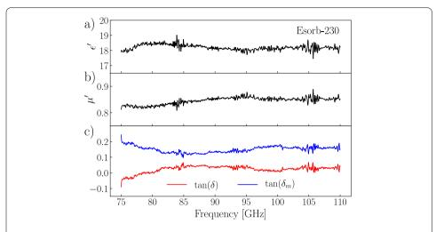
**Figure 6** Electromagnetic parameters of the Esorb-230 material in the frequency range from 75 to 110 GHz. (a) Real part of the relative dielectric permittivity. (b) Real part of the relative magnetic permeability. (c) Dielectric and magnetic loss tangents
