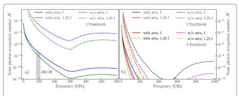
**Figure 9** Estimates of the noise photon occupation numbers for the UT086SS-SS coaxial cable (**a**) and UT047SS-SS and UT034SS-SS coaxial cables (**b**). The estimation does not take into accout the temperature dependence of the attenuation, and the lines represent the lower bounds of the noise photon occupation numbers
