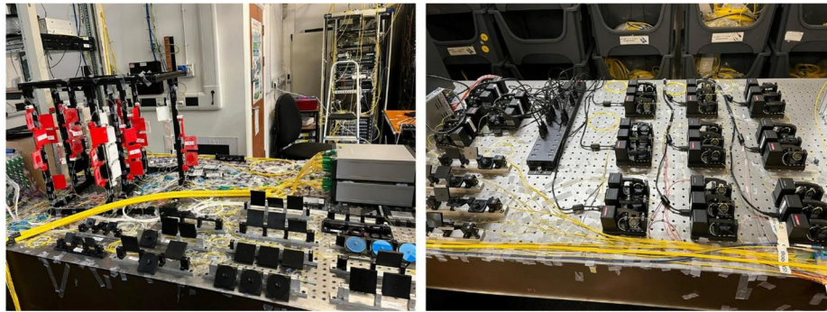
Figure 3 Left: Photography of a part of the experimental setup with manual polarization controllers, Right: Photography of a part of the experimental setup with motorized polarization controllers
