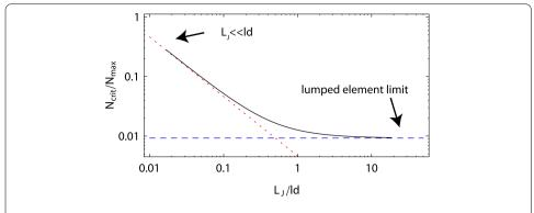
Figure 7 Validity of the quartic approximation. Ratio  $N_{\rm crit}/N_{\rm max}$  according to Eq. (40) (black), in the lumped element limit (dashed blue) and in the limit of small participation ratio  $L_J \ll ld$  (dotted red) for the parameters  $\{\tilde{\omega}_0/2\pi,Q\} = \{7 \text{ GHz},1,000\}$ .
