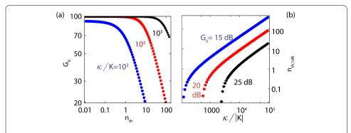
**Figure 4 Dynamic range of the JPA.** (a) Gain  $G_0$  as a function of the photon number  $n_{\rm th}$  of the input signal field for the three indicated ratios  $\kappa/|K|$ . (b) 1 dB compression point as a function of  $\kappa/|K|$  for various gain values  $G_0$ .
