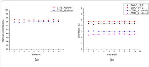
Figure 5 (a) Interference contrast corresponding to "CTRL-X" operation. (b) Error rate under different classical operations
