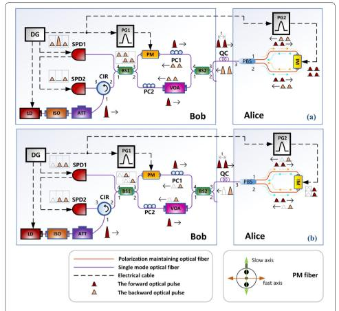
**Figure 4** (a) The forward and backward optical path of the "CTRL-X" operation. (b)The forward and backward optical path of the "SWAP-x-Z" ( $\mathbf{x} \in \{01,10\}$ ) operation. ISO: isolator, PC: polarization controller, VOA: variable attenuator, PG: electrical pulse generator
