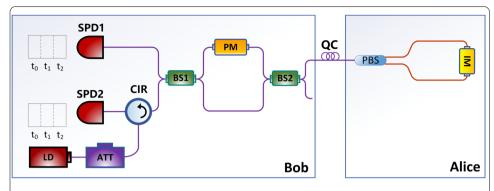
**Figure 2** The scheme based on the Mirror protocol with time-phase encoding. LD: laser diode, ATT: attenuator, CIR: circulator, BS: beam splitter, PM: phase modulator, IM: intensity modulator, PBS: polarization beam splitter, QC: quantum channel, SPDs (SPD1 and SPD2): single photon detectors
