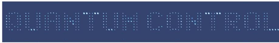
**Figure 1** A BEC “printer”: The robust and versatile control of a BEC allows for producing experimentally lines of points made up of atomic clouds, with which letters and words can be formed
